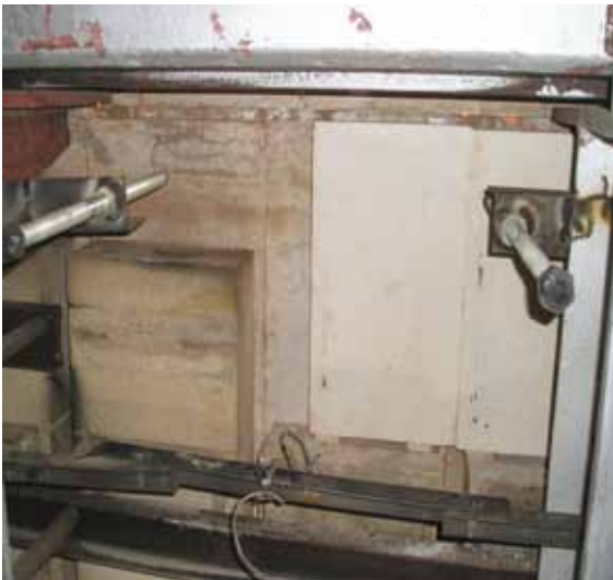
Positioning of metal line over-coat tiles.
